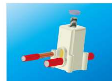
4. 揭开透明盖拧松螺钉,装入分支线后拧紧螺钉,盖上透明盖即可 Pop the transparent top cover, loosen position screw, insert branch cable, tighten position screw, and finish by re-attaching the top cover
